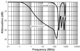
\*measured on Agilent/HP8753ES analyzer
